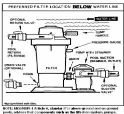
Though the pump is designed for outdoor use, it is strongly advised to protect the electrical components from the weather. Select a welldrained area, one that will not flood when it rains. Pump motors
