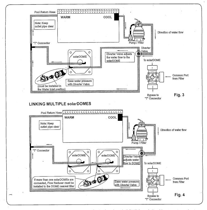
NOTE: The connections in Fig. 3 & 4 show the water flowing into the solarDOME through the side connector and out through the center connector located on the underside of the solarDOME. This diagram is for reference only as the flow may be reversed if you choose.
